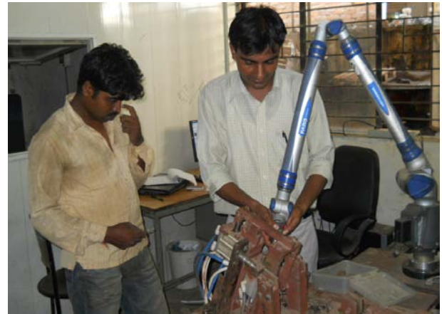
Taking precise measurements of small components with the FaroArm
